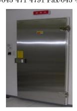
ECCOSHIELD MAS Dooor with Magnetic Area seal is an RF shielded door which is unique in RF sealing, and which is free of the deficiencies of finger stock. Magnets apply pressure over a broad area of a shielding membrane to make doors or removable panels self-sealing with no mechanism, no effort, no maintenance.
